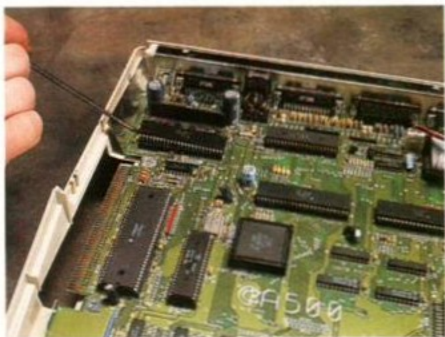
The shield has to be twisted slightly to physically get a grip on the Denise chip, but it bends back to shape without any fuss.
